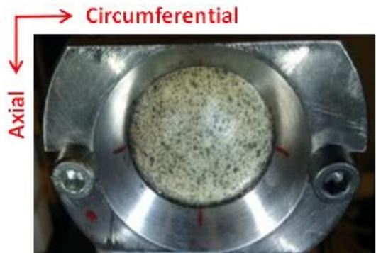
c) Inflation test device. Speckle pattern is made before starting the inflation test
