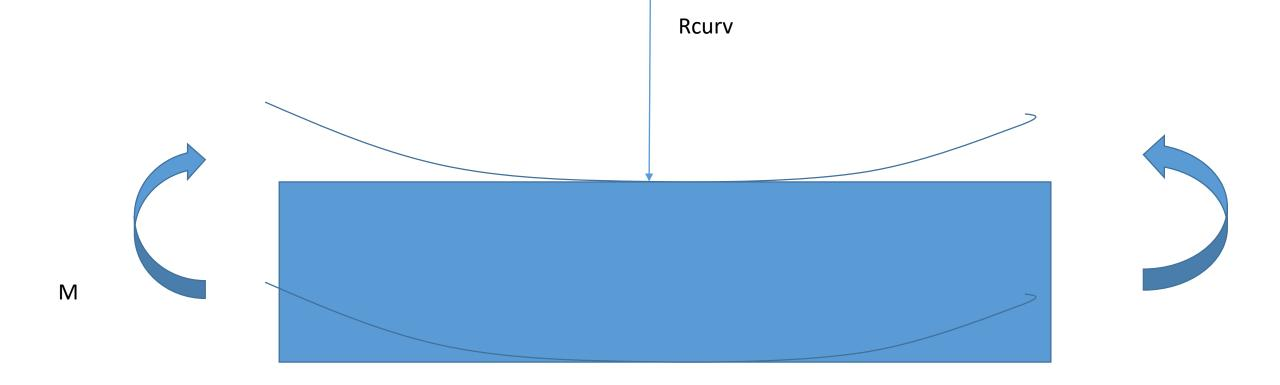
The bending moment => curvature of the beam
