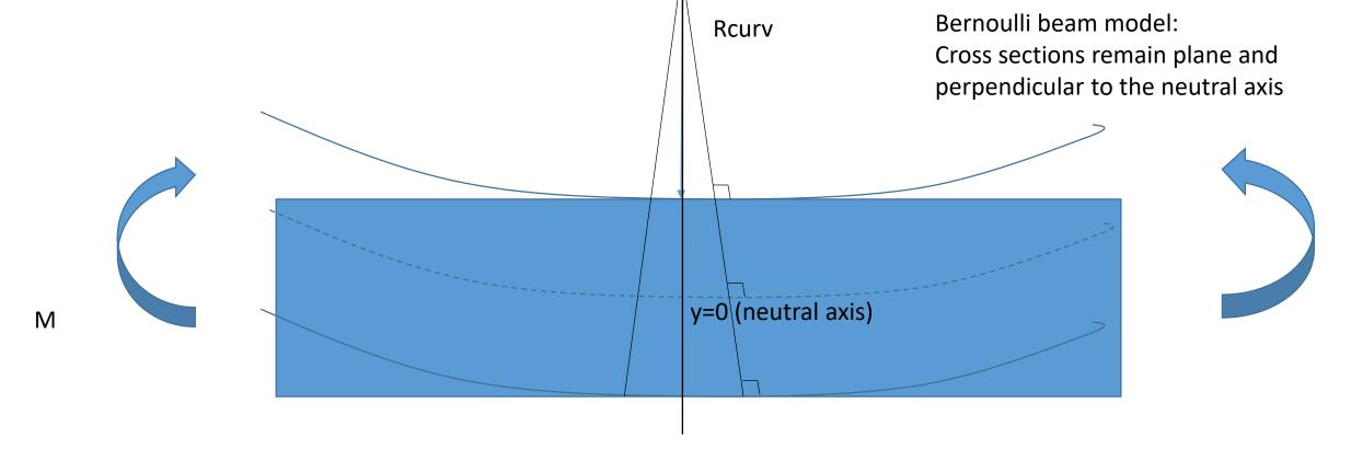
The bending moment => curvature of the beam
