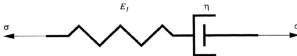
Total strain = spring strain + dashpot strain:
